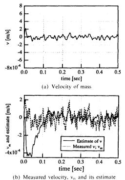
Fig. 5 Stabilization performance obtained by adding a friction compensator based on the friction observer 2
