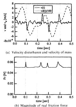
Fig. 3 Stabilization performance obtained by the feedback controller alone
