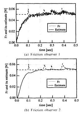
Fig. 4 Estimation performances of two friction observers in the noisy environment
